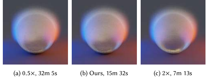
Fig. 5. Step-size ablation with render time shown under each image. We multiply the adaptive step size by a constant factor before applying the unchanged clamp \Delta_{\min} . A conservative 0.5\times step size produces a result nearly indistinguishable from our default. A doubled step size, however, introduces visible differences because overly aggressive marching can skip zero crossings.
