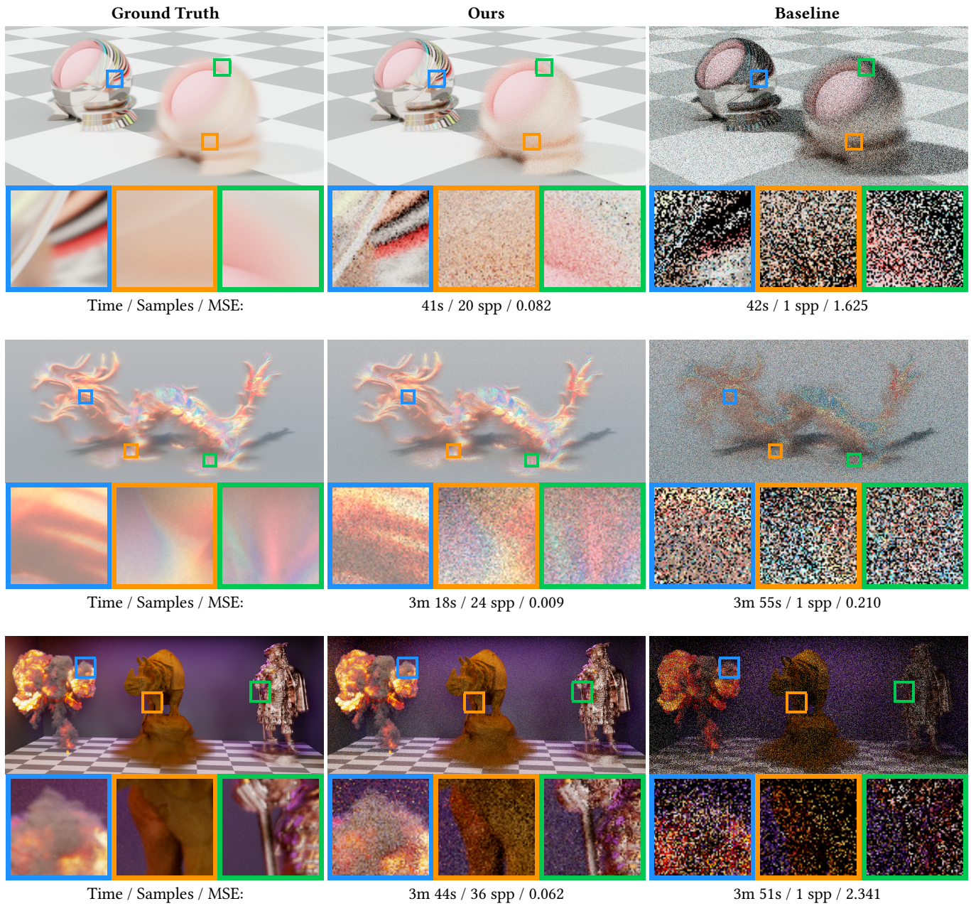
Fig. 6. We evaluate our GPIS-ray intersection method in a path-tracing renderer, comparing it to the baseline method across multiple scenes with various types of covariance functions. We render each scene with both methods at equal time, using the same renderer and scene settings. Our method enables more samples per pixel in the same time budget, resulting in significantly lower image noise.
